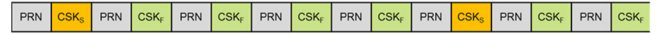
Fig. 2. Scheme for the insertion of slow and fast bursts in the PRN sequence.
