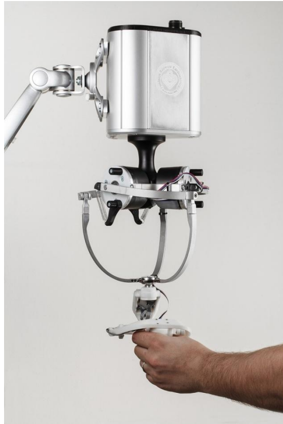
Figure 6 Input device, based on a delta robot design
