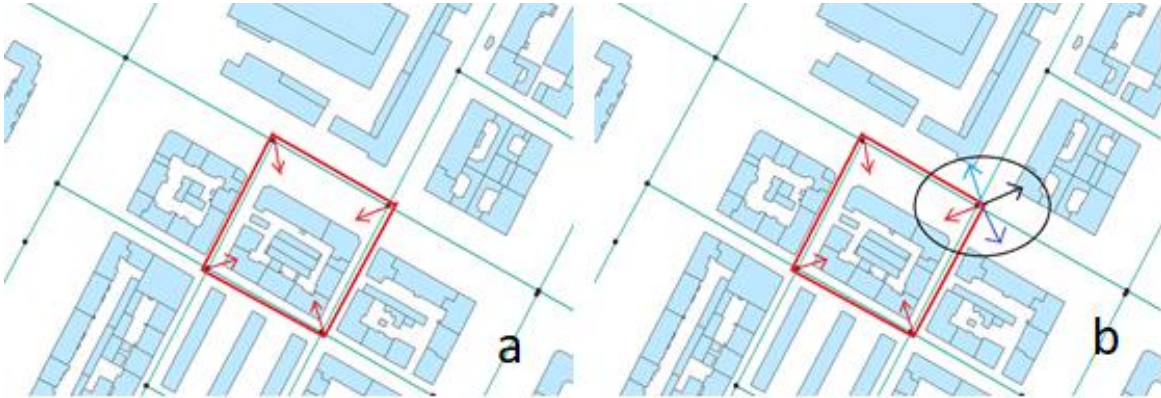
Figure 4 (a) Water demand q_{j,w} for the mesh element w , (b) Water demand for the i -node.
