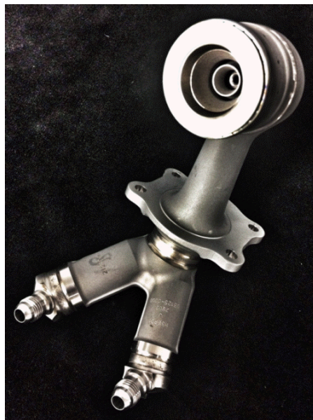
Figure 4. LEAP engine fuel nozzle produced by GE aviation (with the Courtesy of GE reports [24]).
