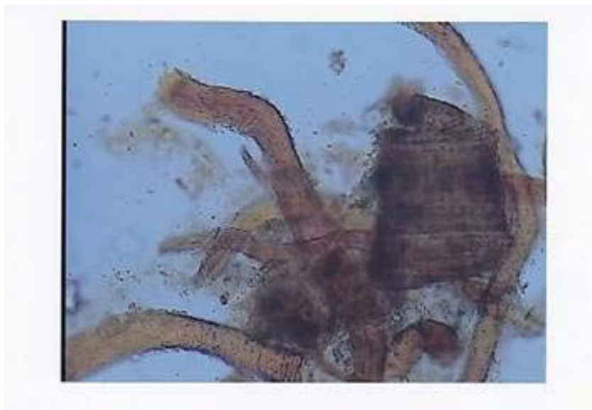
Figure 6. Optical micrograph (200X) of hydrolyzed wool from test 2.
