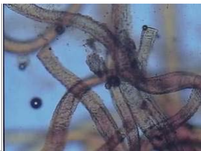
Figure 7. a) Greasy wool uncompressed and well impregnated with water prior to hydrolysis and b) hydrolyzed wool after hydrolysis in test 3
