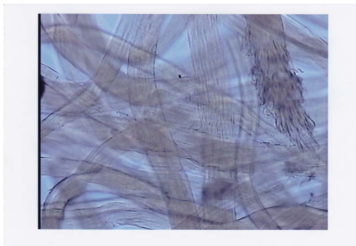
Figure 14. Optical micrograph (100X) of hydrolyzed wool from test 170 °C, density 350 kg/m 3 , liquor ratio 1:3 and time 60 min.
