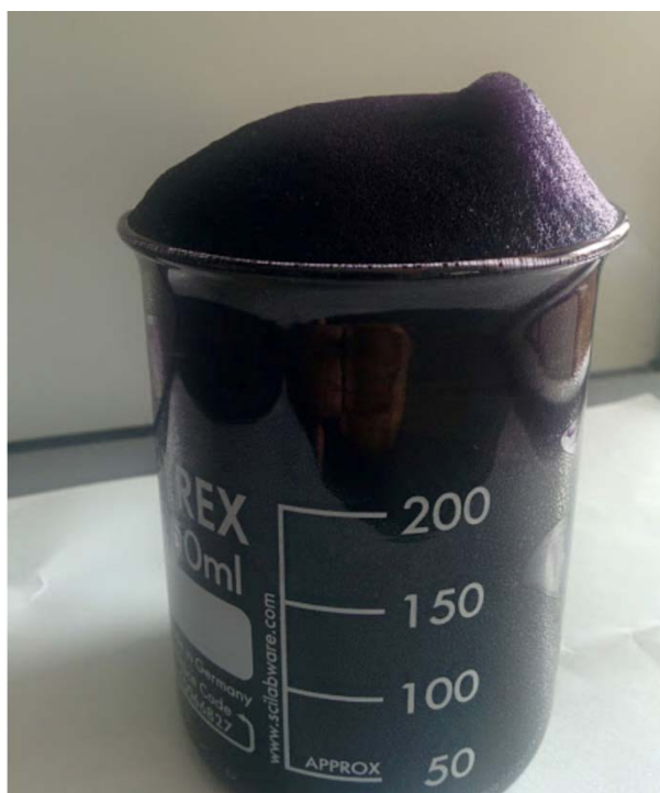
Figure 4. Representation of foam produced from keratin hydrolyzate along with dye auxiliaries.
