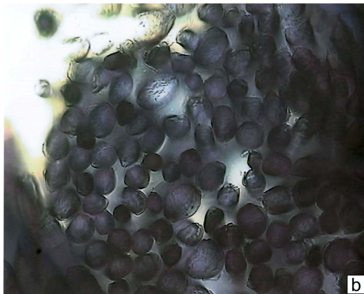
Figure 9. Optical micrograph (100X) of fiber cross sections of wool a) conventional dyed and b) foam dyed.
