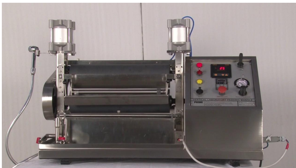
Figure 6. Universal padding mangle Matis (Switzerland).
