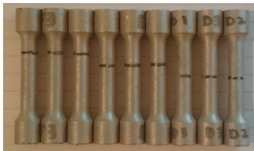
Figure 10. Customised specimen set failure points.
