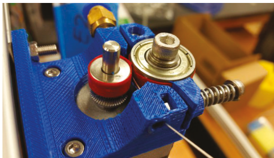
Figure 10. Wire feed Bowden assembly assembled with supplementary hardware and “Compact Bowden Extruder thing: 275593”. Note that a common 1.75 mm extruder drive tooth gear has been inverted and coupled with electrical tape to provide frictional rolling resistance to aid in guiding the 1100 series aluminum wire.
