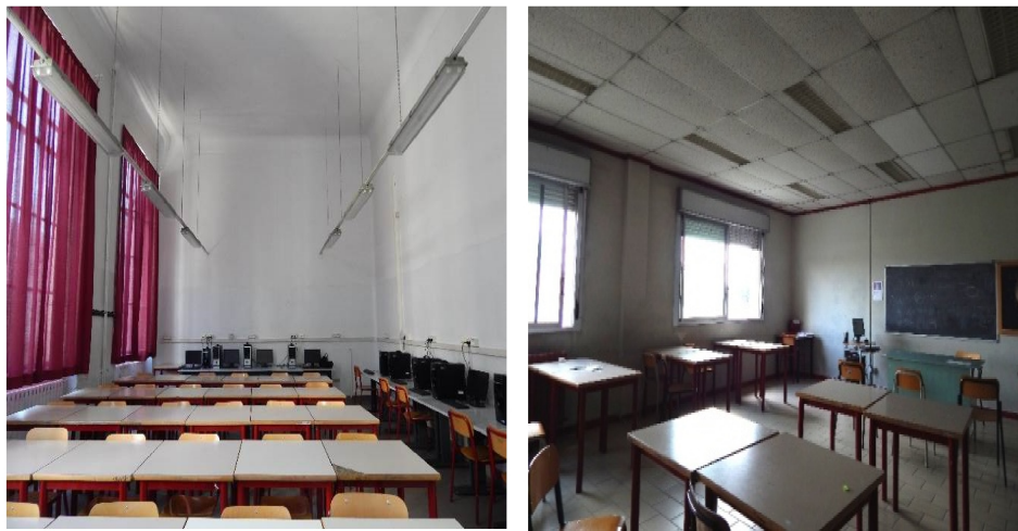
Fig. 2.2 Left side: a huge volume classroom, with high ceiling and no absorbing surfaces of school A; right side: a classroom with limited volume and absorbing ceiling of school B.
