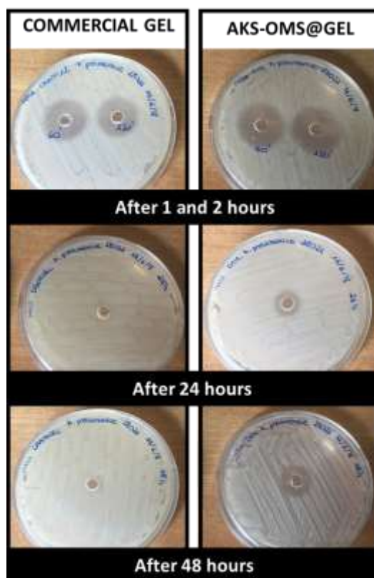
Figure 7.10 Disk-diffusion method of the AKS-OMS@GEL in comparison with the amikacin-based commercial gel with using K. Pneumoniae as test microorganism.
