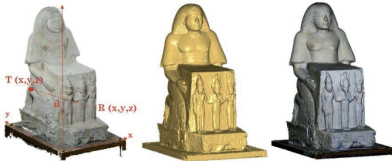
Figure 2. Photogrammetric point cloud, mesh and textured mesh.
