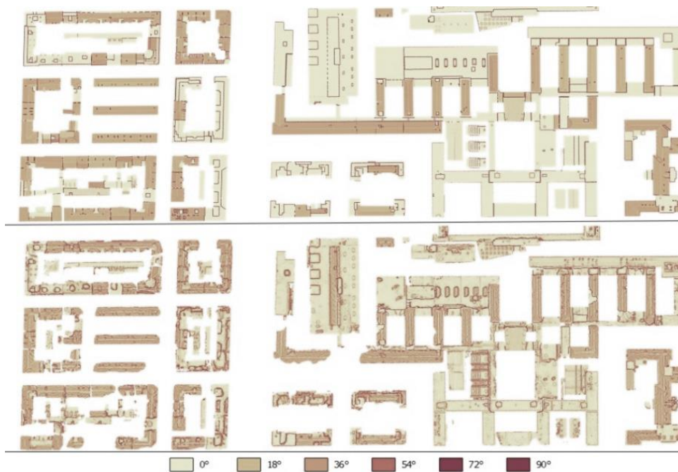
Figure 10: Slope analysis with manual DSM (upper) and MicMac DSM (lower)
