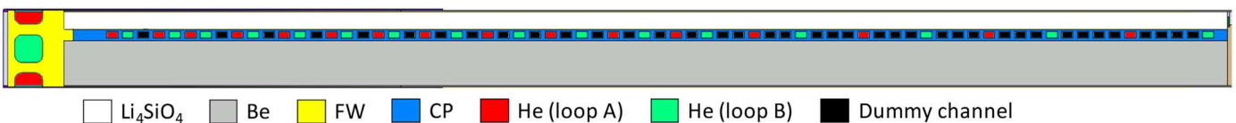
Fig. 4. Radial-poloidal cross section of a HCPB BM, showing the different materials and highlighting the channels of loops A and B, as well as the dummy channels in the CP.
