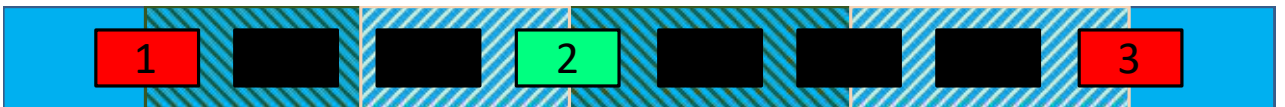
Fig. 6. Cross section of a CP, showing the split of the solid volume between adjacent channels, in the two possible cases: when the number of dummy channels between two active channels is even or 0 (as for channels 1-2), and when it is odd (as for channels 2-3). The color code is the same as Fig. 4.
