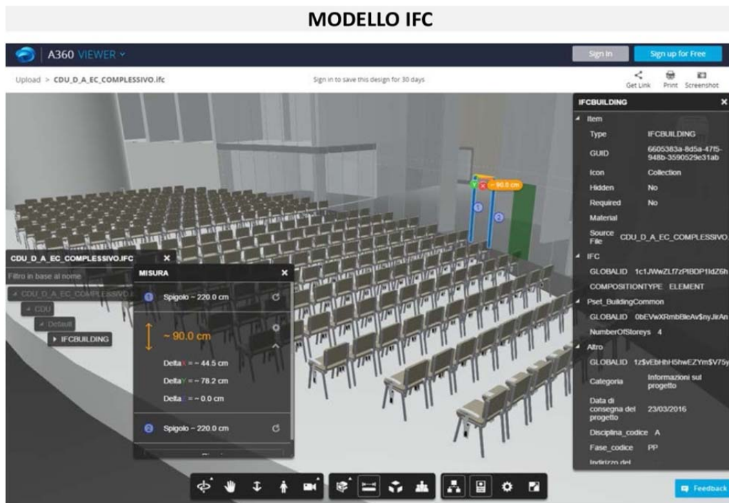
Figure 77: BIM model visualization through IFC viewer. Case study: UnipolSai headquarters, Milan.
