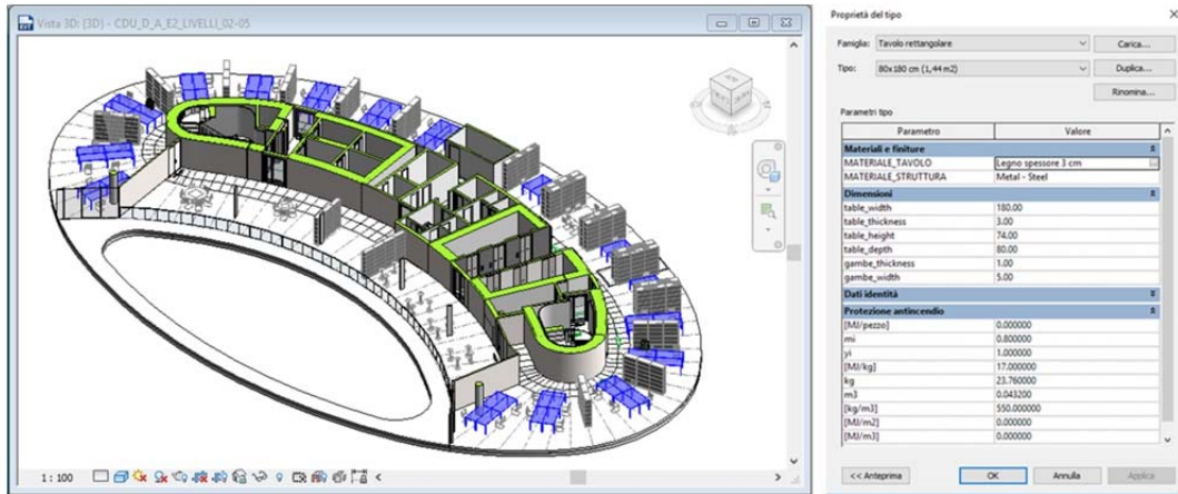
Figure 72: Desk parameters for specific fire load calculation.
