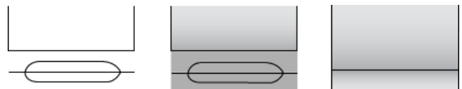
Fig. 8. The street graph (left) leads to unwanted geometries (center). A simplified graph can solve the problem without changing the current algorithm (right).
