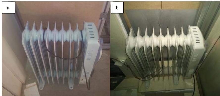
Fig. 5. (a) Configuration A (bulk wall); (b) Configuration B (wall coated with low-E paint)
