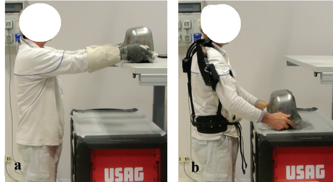
Fig. 3. Repeated manual material handling task: (a) without exoskeleton; (b) with exoskeleton.
