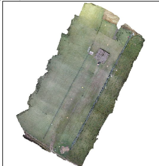
Figure 12. The georeferenced dense point cloud of the flight field, obtained by the image processing by the tool Agisoft Photoscan Professional.
