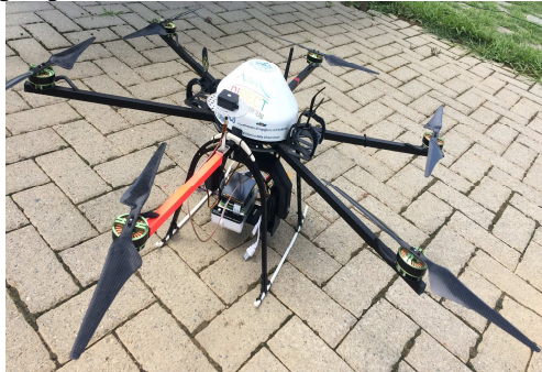
Figure 1. The employed multi-rotor platform used for the image acquisition
