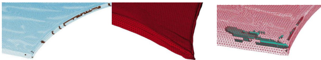
a. Outer face-sheet cracking b. Foam core compression c. Foam failed elements
