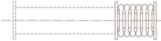
Figure 3.10: Axial collapse mode [1]
