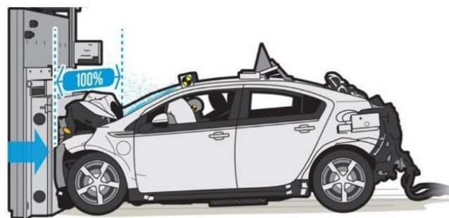
Figure 3.4: Schematic of full frontal crash test
