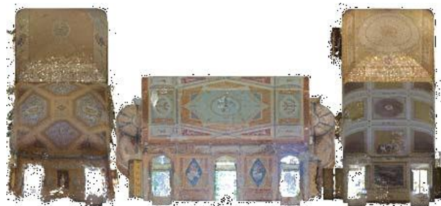
Figure 6. Point clouds of the five main room in the lower floor of Palazzo Sarmatoris .
