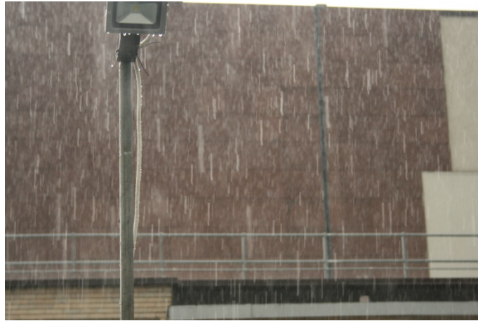
Figure 5.11 - Image acquired at 16:25 on 14/05/2016 in correspondence with the peak of intensity of the event. The presence of overlapped drops causes the missed recognition and, as a consequence, an underestimate of the rainfall intensity
