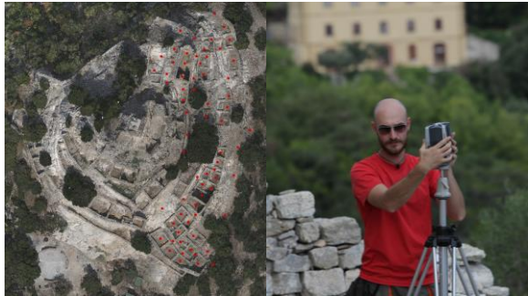
Figure 9. TLS acquisitions (right) and scans position (left)
