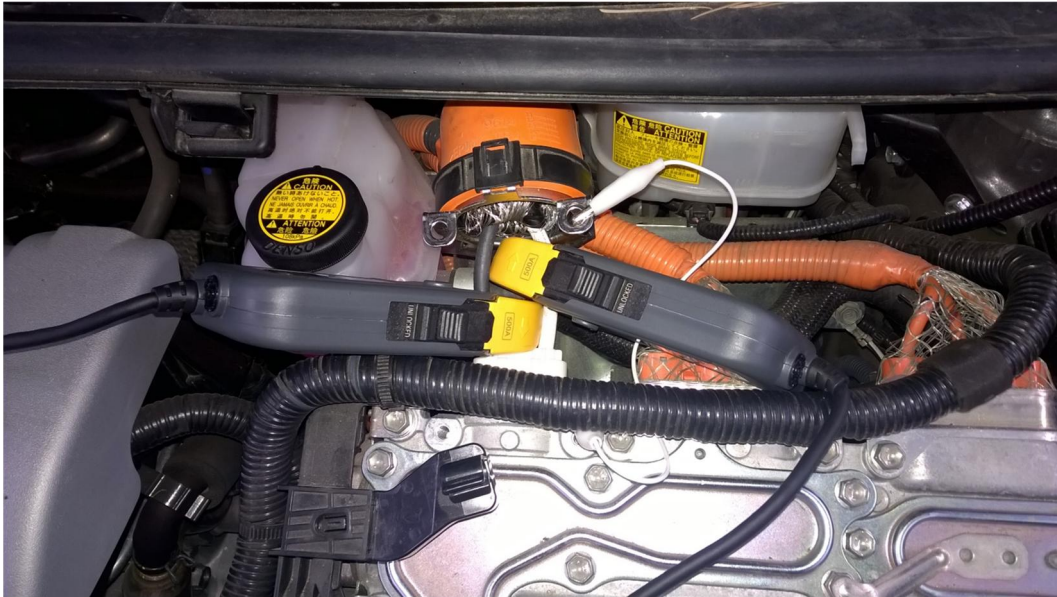
Figure 25: Yaris Hybrid – Detail of current clamp positioning
