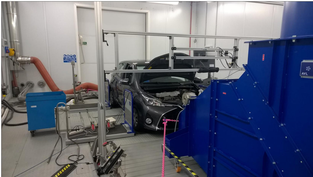
Figure 22: Climatic chamber and chassis dynamometer at VELA 8 lab
