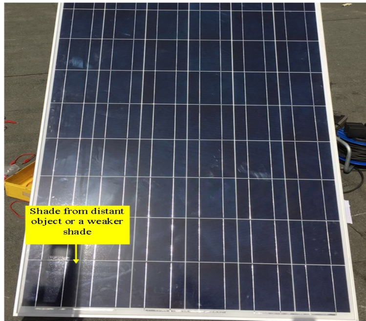
Fig. 2.11 Partial shading caused by a distant object.
