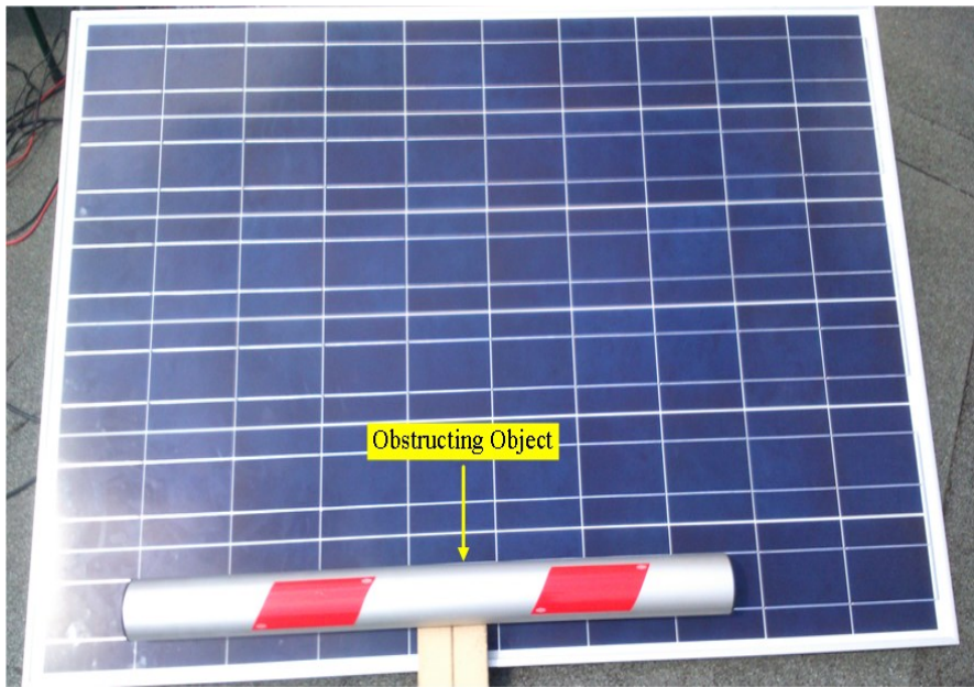
Fig. 2.13 Partial shading caused by object close to the surface of the PV panel.
