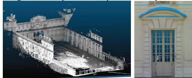
Figure 6 General view of the realized TLS survey (left), zoom on the acquired windows (right).
