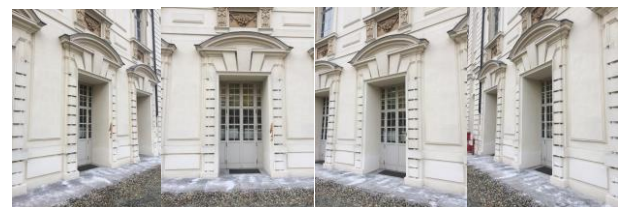
Figure 3. Part of a dataset acquired by a Canon 600D with a 18 mm (shooting distance= 3 m; GSD= 0.7 cm )
