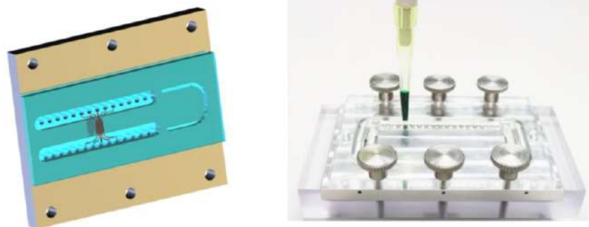
Fig. 3.5 Picture illustrating the five channel functionalization flow cell. The Polydimethylsiloxane (PDMS) flow cell (blue) with the five fluidic channels (red) attached to an aluminum plate (left). Filling of a channel flow cell using a standard microliter pipette (right).
