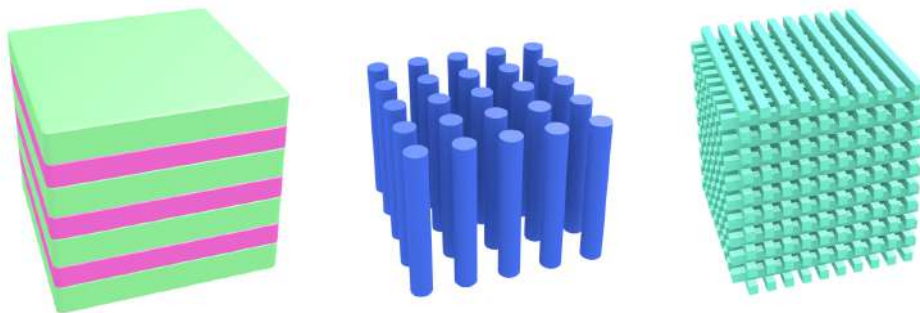
Fig. 1.1 Simple examples of one, two, and three dimensional photonic crystals. The different colors represent materials with different dielectric constants. The defining feature of a photonic crystal is the periodicity of dielectric material along one or more axes.
