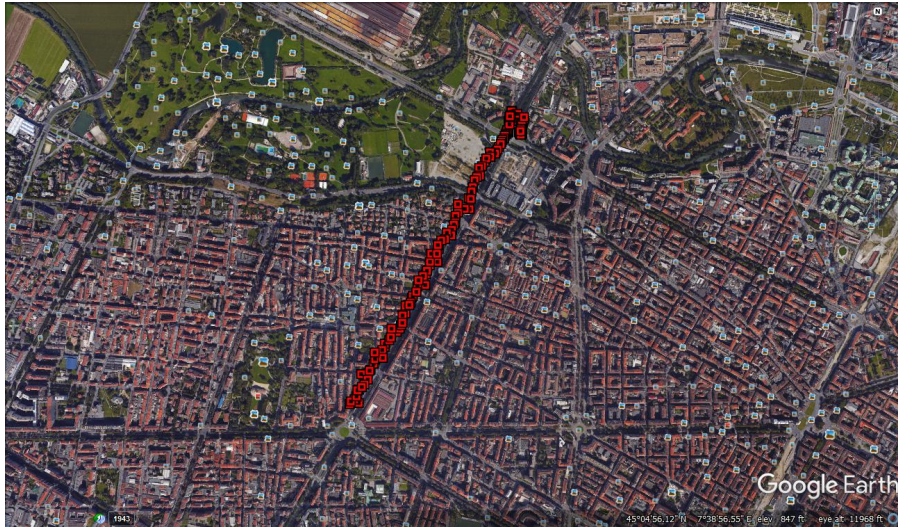
Fig. A.4 Example of a dynamic urban data collection, obtained in downtown Turin, Italy. Position solutions are shown with red squares.
