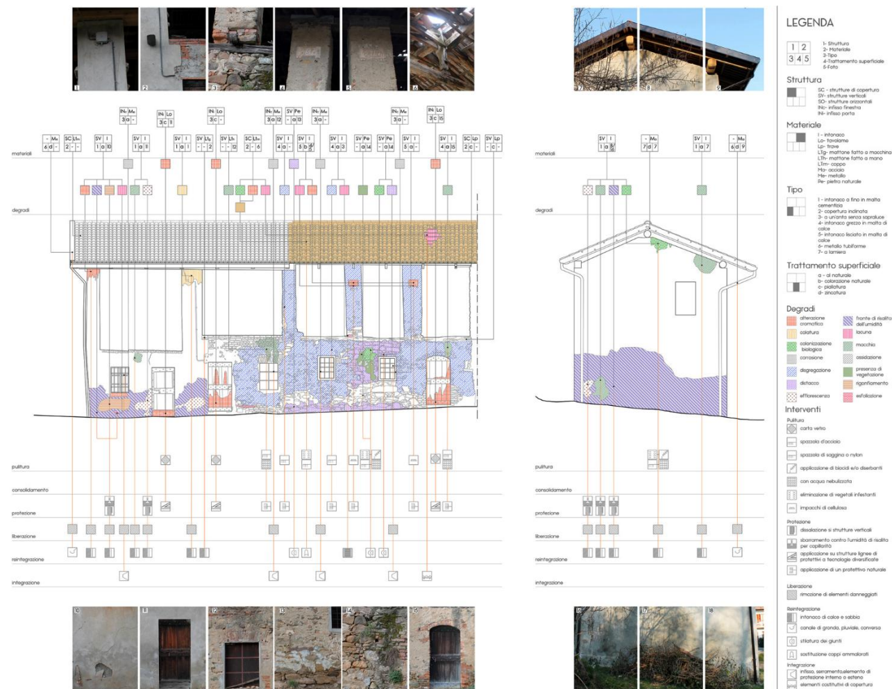
Figure 1. Example of a restoration project: from the analysis of materials and decays to the interventions' proposal
