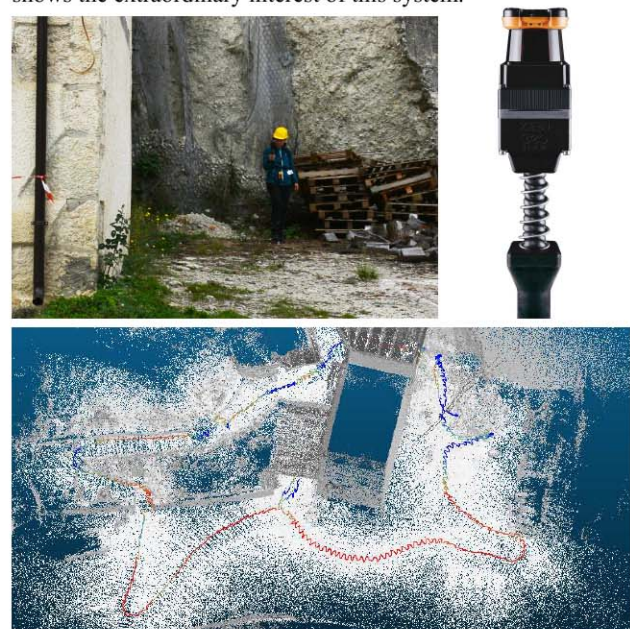
Figure 4 Zeb 1 by Geo-Slam: an acquisition moment (left), the instrument (right). (Down) Geo-Slam path, with quality of registration attribute in scalar colour
