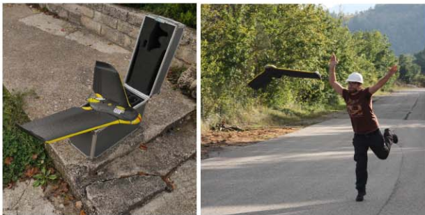
Figure 5. eBee platform (left), take-off phase (right)
