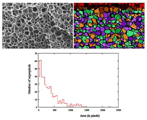
**Figure 11:** An image of microcellular plastic and its segmentation. (Microcellular Plastic Micrograph developed at Indian Institute of Technology, Delhi. Courtesy: Gandhi.iitdelhi, Wikipedia, https://commons.wikimedia.org/wiki/File:Cyclic\_Microcellular\_Foam.tif). The area of the image is 600 x 376 pixels. In the lower panel, there is the distribution of the super-pixels.
