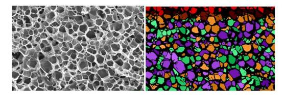
**Figure 9:** The whole micrograph of the Figure 2 and its segmentation. (Microcellular Plastic Micrograph developed at Indian Institute of Technology, Delhi. Courtesy: Gandhi.iitdelhi, Wikipedia). The area of the image is 600 x 384 pixels.
