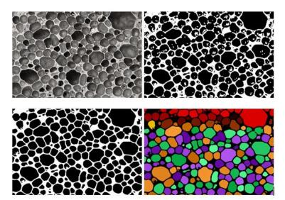
**Figure 6:** In the upper-left panel, we can see a micrograph of a metal foam (Courtesy: metalfoam.net). In the upper-right panel, the corresponding black and white image obtained by using GIMP and its filter Generic-Dilate to enhance the boundaries of the black domains. This filtered
