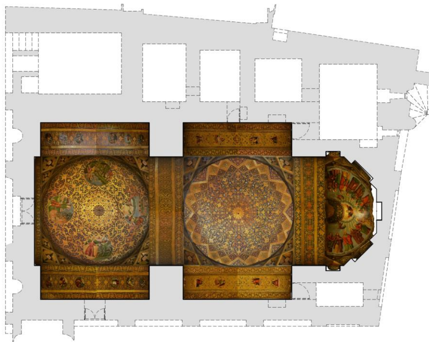
Figure 6. The complete vaults orthoprojections superimposed on the upwards plan.
