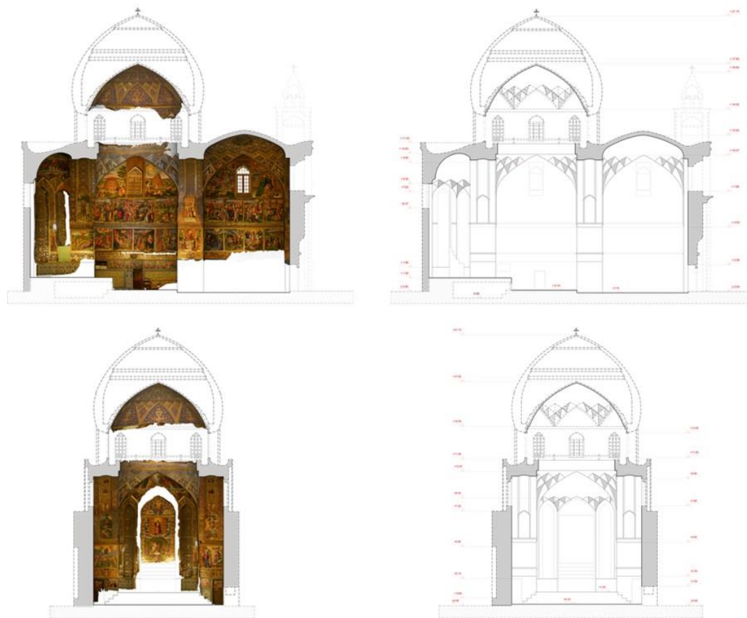
Figure 7. Some examples of 2D architectural drawings with orthoprojections of frescoed walls and vaults.
