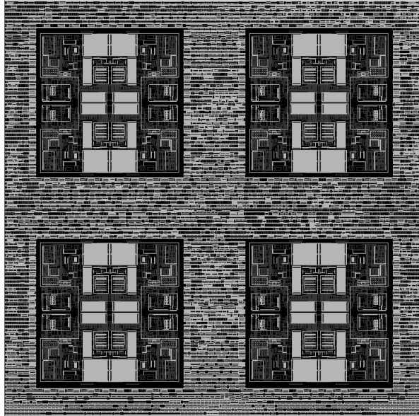
Figure 4: Layout view of a 4 \times 4 pixel region (PR). The design includes 16 analogue front-ends arranged into 2 \times 2 analogue islands surrounded by a common digital logic for data readout and configuration.
