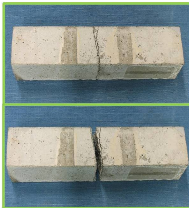
Figure 12. Detail of one of the specimens after the final three-point-bending test, with the creation of a new crack path partially separated from the one generated via the first flexural test.
