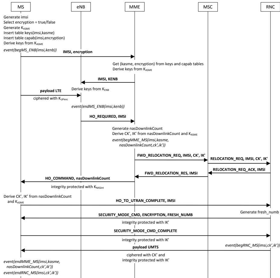
Figure 3: LTE to UMTS handover
