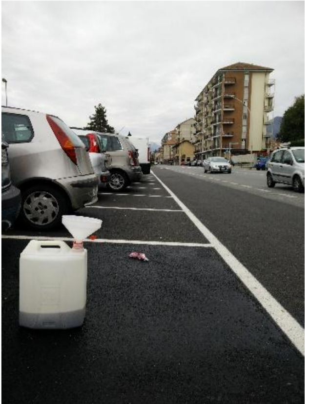
Water collection from a urban pavement for the first and second investigation stages
