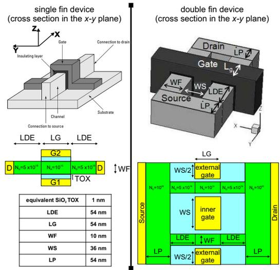
Fig. 2. Single fin DG MOSFET (left) and double fin DG structure (right). Green areas represent Si regions, the light blue SiO<sub>2</sub> and yellow the metal gates.
