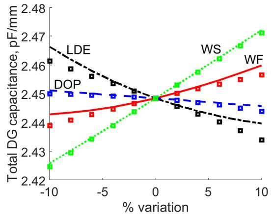
Fig. 7. Drain-gate capacitance of the two-fin DG structure.
