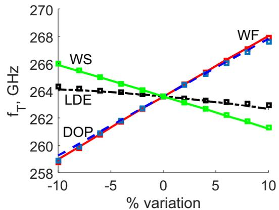
Fig. 8. Cut-off frequency of the two-fin DG device.
