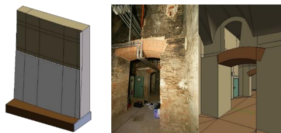
Figure 5. Modeling of the irregular wall in the Castle underground
