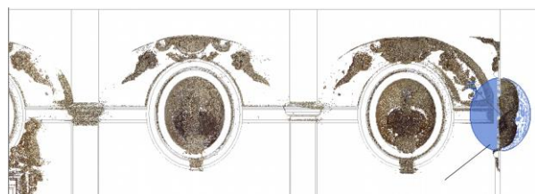
Figure 12. Creation of niche by subtraction solid.
