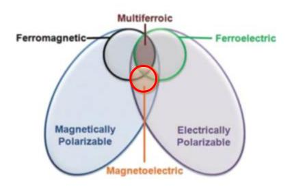
Venn diagram representing the overlap of physical properties in multiferroic materials
