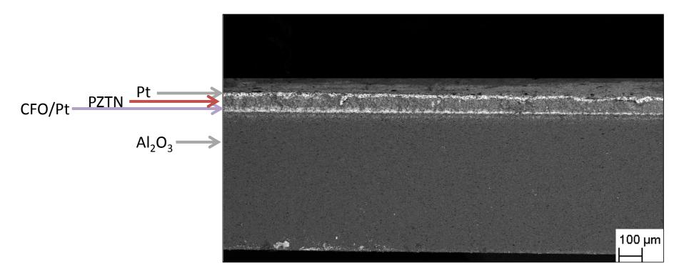
Magnetoelectric composite bilayer films by electrophoretic deposition
