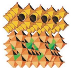
Ferroelectrics crystallize in the **perovskite structure** and it maintain a fraction of the polarisation when the field is removed, after poling
