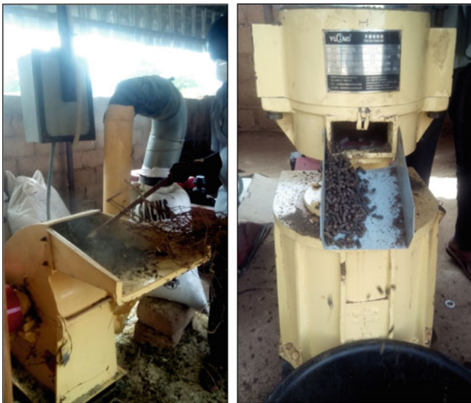
Fig. 15.8 The machines in the pellet making facility. The electric mill ( left ) and the pellet machine ( right )
