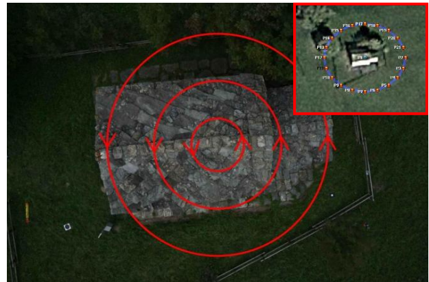
Figure 5. Schema of the circular flight for oblique images acquisition (a screen shot of the Mikrokopter tool is in the top right part of the image)
