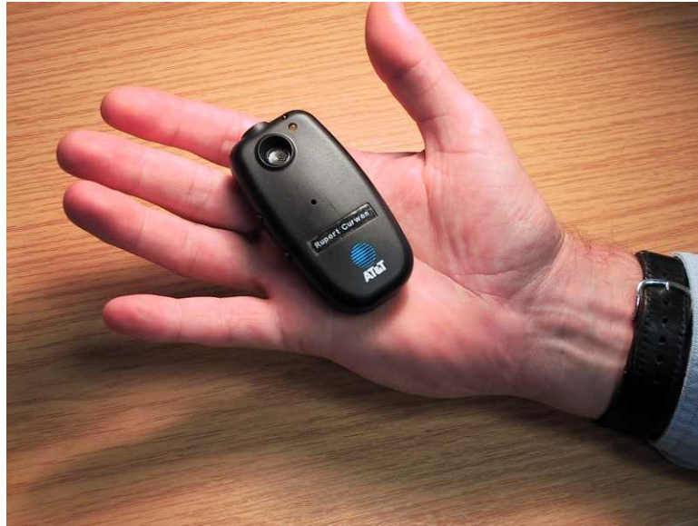
Figure 4.16: The Bat transmitter. Image from http://www.cl.cam.ac.uk/research/dtg/attarchive/bat/ .
