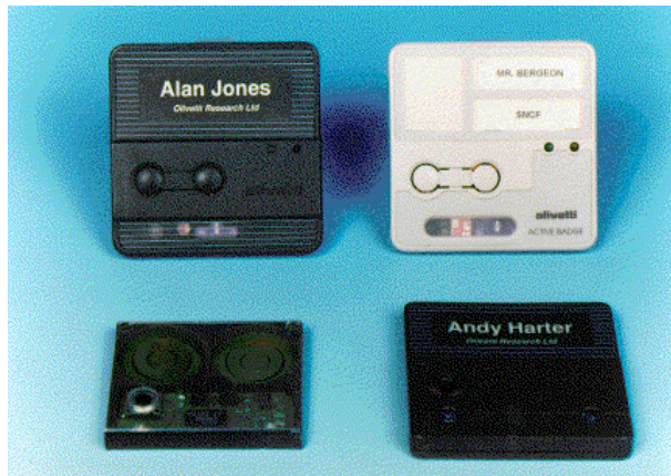
Figure 4.11: The picture shows four generations of the Active Badge. Bottom left, the first version, with a unique five bit code. Bottom right, the second version, with a ten bit code. Top left the third, current, version, with a forty-eight bit code, bi-directional capabilities, and an on-board 87C751 microprocessor.
