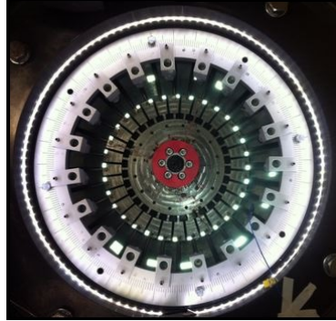
Figure 9: Spinning test rig with 19 permanent magnets.
