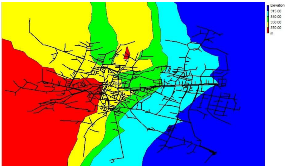
Fig. 1. Scheme of the WDN analyzed in the present work. The colormap represents terrain elevation.
