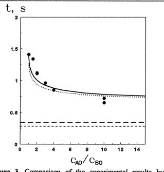
Figure 3. Comparison of the experimental results by Pohorecki and Baldyga (1983) [•] and the predictions of the three-stage micromixing model.
