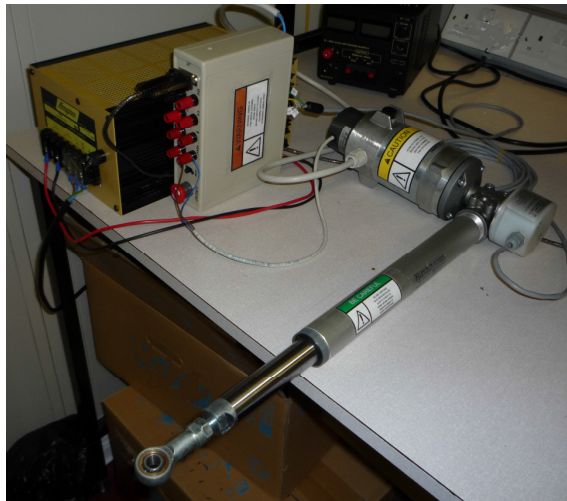
Fig. 3 Complete EMA actuation system
