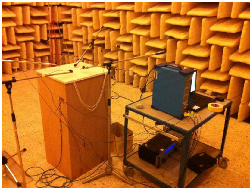
Figure 6.15: Modal sound insulation measurement performed with the scale model in the anechoic chamber. Receiving space microphones are placed randomly at 1 cm from the partition.
