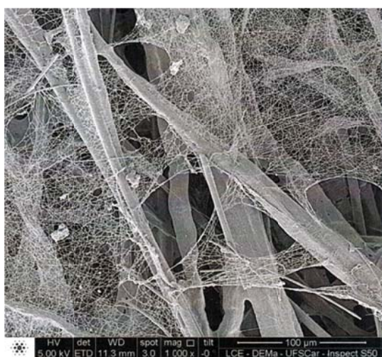
Fig. 1 Nanofiber/cellulosic media, 1000x. Fig. 2. 20000x image, showing nanofiber details.
