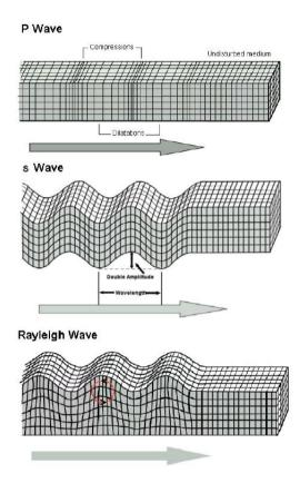
Figure 1.3: Wave propagation modes in an elastic medium.
