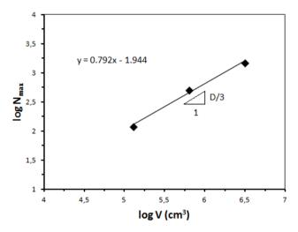
Figure 4.8: Volume effect on N<sub>max</sub>.
