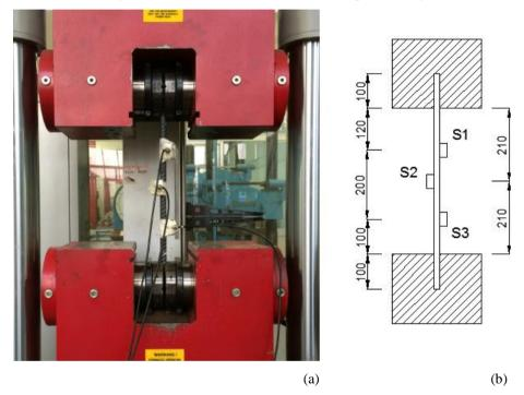
Figure 3.3: Tensile test: (a) experimental test; (b) schematic representation of the experimental setup. S1, S2 and S3 are the sensors applied to detect the AE signals.
