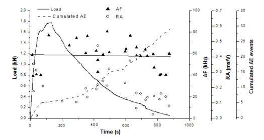
Figure 3.15: Specimen B2 (1190x200x100 mm): load vs. time curve, AF and RA values of the detected AE events, and cumulated diagram of the AE events. The straight line represents the linear regression of the AF values during the test.
