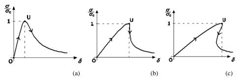
Figure 2.6: Stress vs. displacement response of a specimen in compression: (a) normal softening; (b) vertical drop; (c) catastrophic softening (snap-back).
