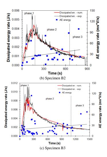
Figure 3.28 (a),(b),(c): Energy dissipation rate and AE energy rate as a function of time for the three specimens.
