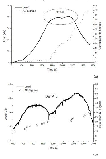
Figure 4.3: (a) load vs. time curve and cumulated diagram of the AE events. (b) Detail of load vs. time curve, and AE cumulated number in the vicinity of the peaks load.
