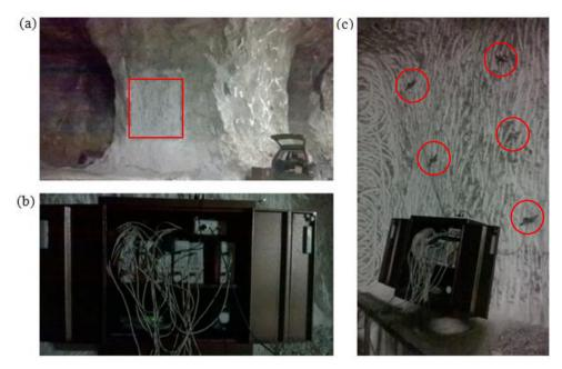
Figure 4.4: (a): hole 4x4 m without detensioned surface layer; (b,c) AE Monitoring set.
