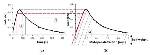
Figure 3.25: Sketch of the procedure followed to compute the dissipated energy rate: (a) load-time and (b) load-displacement diagrams.
