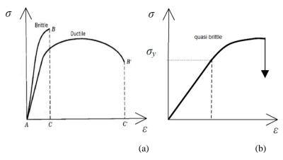
Figure 2.1: (a) brittle and ductile behavior; (b) quasi-brittle behavior.
