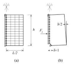
Figure 2.12: (a) Scheme of finite element mesh (b) scheme used for calculation of elastic coefficients.
