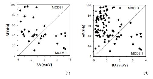
Figure 3.31: Fracture mode identification by means of the relationship between RA and AF values for a concrete specimen under compression: (a) from 0 to 1000 s; (b) from 1000 s to 2500 s; (c) from 2500 s to the end of the test; (d) total duration of the test.
