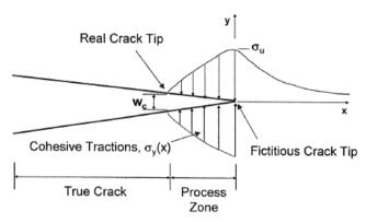
Figure 2.9: Cohesive Crack Model.
