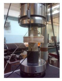
Figure 4.2: AE piezoelectric transducer positioned around the monitored gypsum specimen.
