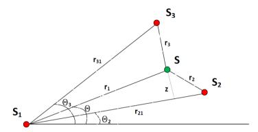
Figure 1.8: AE source and sensors: Polar coordinates system.
