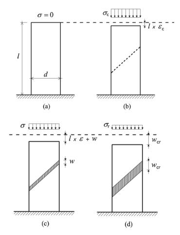
Figure 2.5: Subsequent stages in the deformation history of a specimen in compression.
