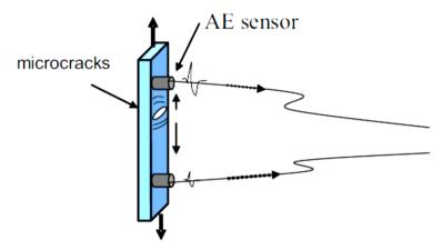
Figure 1.2: Principle of AET: stressed material generating an elastic wave.
