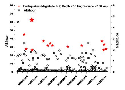
Figure 4.6: AE rate compared to local seismic activity.
