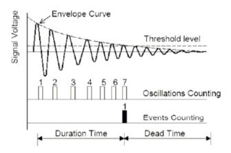
Figure 1.5: Counting methods for AE events: oscillation (ring-down) counting and event counting from an AE waveform.
