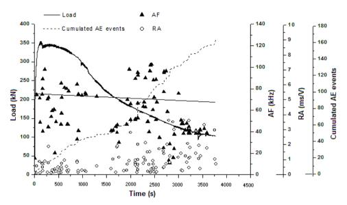
Figure 3.30: Compression test: Load vs. time curve, AF and RA values of the detected AE events, and cumulated diagram of the AE events. The straight line represents the linear regression of the AF values during the test.
