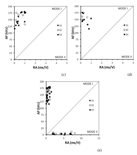
Figure 3.9: Fracture mode identification by means of the relationship between RA and AF values for a steel specimen under tensile: (a) from 0 to 16 s; (b) from 16 s to 31 s; (c) from 31 s to 139 s, (d) from 139 s up the end of the test; (e) total duration of the test.
