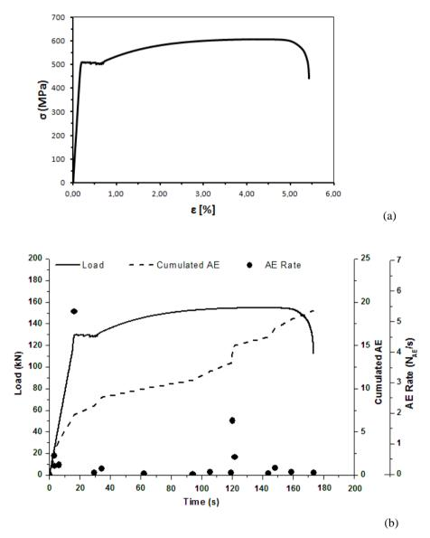
Figure 3.4: (a): stress vs. strain diagram; (b): load vs. time curve, cumulated AE events and AE counting rate diagram.
