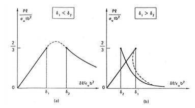
Figure 2.8: Load–deflection diagrams: (a) ductile; (b) brittle condition ( $\delta_l = \lambda^3/6$ ;  $\delta_2 = s_{E,l} \lambda^2/2 \varepsilon_u$ ).
