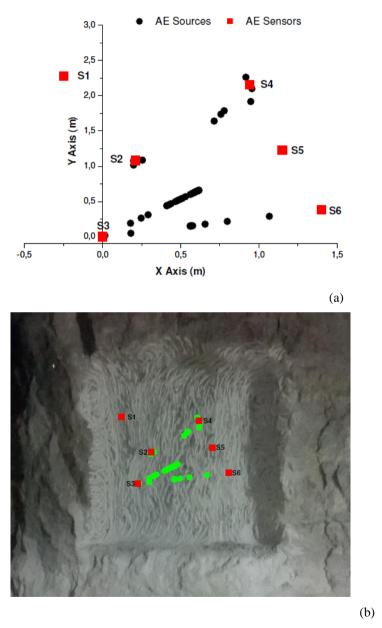
Figure 4.7: (a) AE source localization (b) preferential crack propagation.
