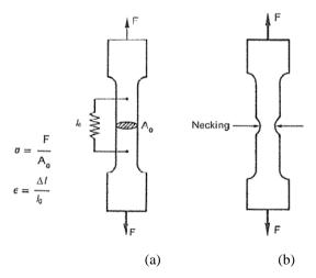
Figure 2.2: (a) uniaxial tensile test; (b) necking phenomenon.
