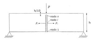
Figure 2.10: nodes of the finite elements pattern disposed along the crack propagation line.
