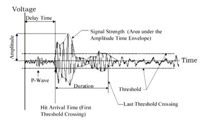
Figure 1.4: AE signal and its main parameters.
