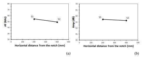
Figure 3.19: Specimen B3 (1450x300x150 mm): (a) mean value of the AFs and (b) average amplitude of the signals detected by the two sensors during the test.
