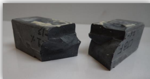
Figure 6.3 Typical fracture planes of plain (a), GNP_3 (b) and CBF (c) reinforced cementitious composites after 3-point bending test
