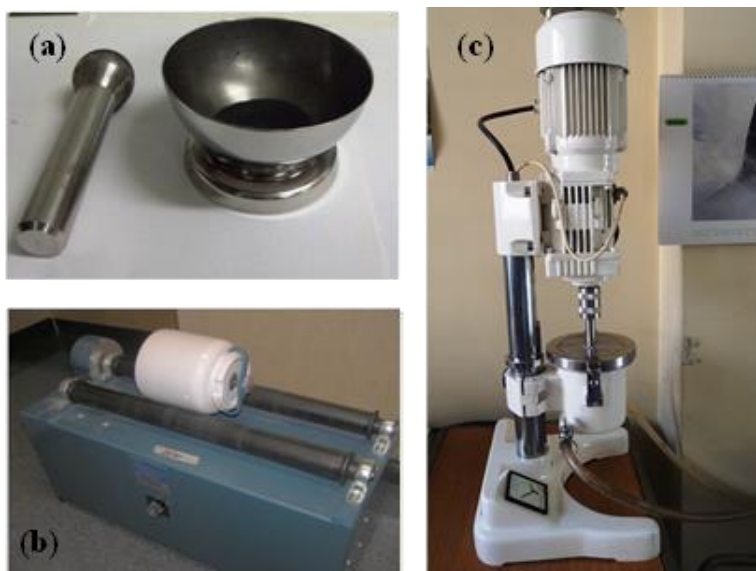
Figure 1.15: Grinding apparatus (a) mortar and pestle, (b) ball mill, (c) attrition mill
