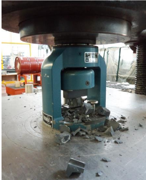
Figure 1.19: Compression test setup of cement paste composites
