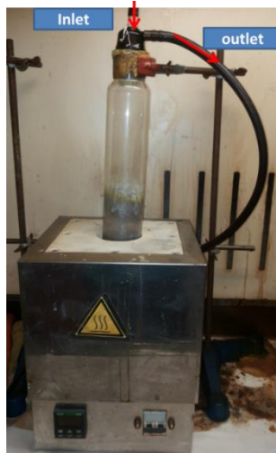
Figure 1.11: Experimental setup for the pyrolysis of organic raw materials
