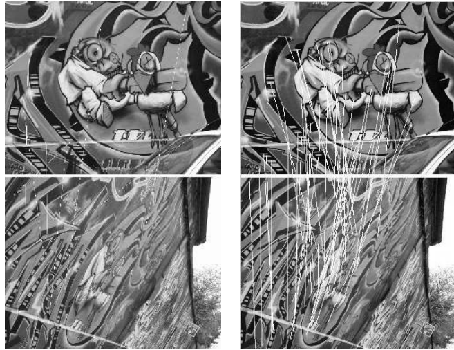
Figure 1.9. Feature matching comparison [23]. In the figure, SIFT (shown), Harris-Affine, Hessian-Affine and MSER(shown) find 2, 3, 1 and 42 correct matches.
