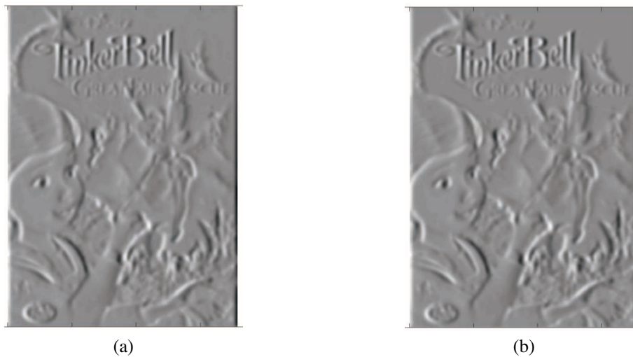
Figure 4.2. Gradient of vertical direction. (a) is generated by Gaussian gradient operation. (b) is generated by Gaussian blurring and adjacent pixels difference.
