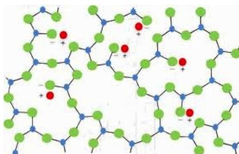
Figure 5.32 Sodium silicate gel chemical structure after gelation.
